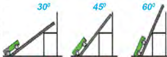
Fig. 8.7: Inclined planes with the same height but different slopes
