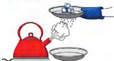
Fig. 1.5 Observation of evaporation and distillation
