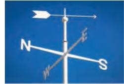
The tool is placed on top of a weather station and gives accurate results about the direction of the wind which provides a lot of information about the changes that take place in the weather.
