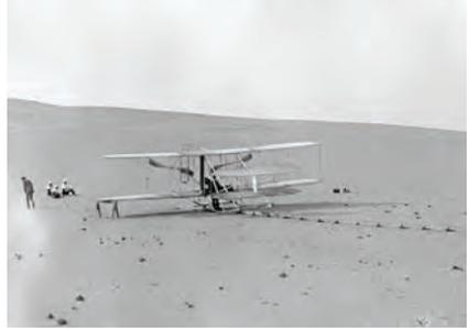
During the 1901 glider tests, the Wright brothers had discovered that "wing warping" created unequal drag on the two wings. The key to solving the control problem was the addition of a rudder to the glider design in 1902. They developed a direct linkage between the rudder and warping system. With the success of this system design, the Wrights were ready to move onto a powered aircraft.
