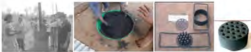
Fig 9.11: steps to form a carbonized briquette
