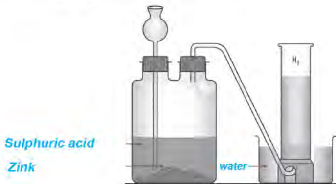
Figure: 16.2 laboratory preparation of hydrogen gas
